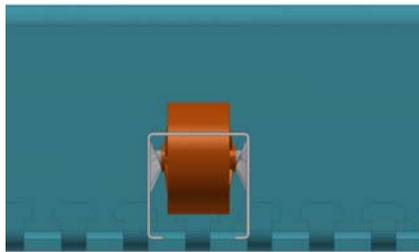
Install roller track by squeezing the bottom of each piece and inserting into the teeth of the front and rear members as shown.
