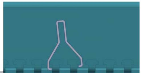
Install guide or lane dividers by opening or “flexing” of each piece over two teeth of the front and rear members as shown above.
