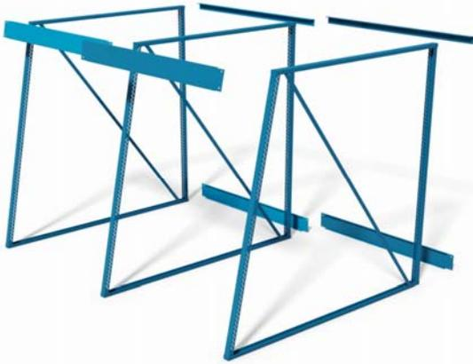
Locate the Angle Brace and the Sway Braces. Bolt the Sway Braces to the top front and bottom rear of frame and the Angle Brace to the top rear of Vertical Frame.
